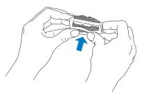
4 Keeping your hand away from the blast doors, place the cartridge into the front of the CEW, until is it approximately 90 percent inserted.
